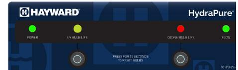
Solid red OZONE BULB LIFE indicates Lamp is not powered on. Bulbs and ballast should be inspected for proper connection prior to replacement. See page 13
