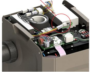
5 Carefully lift the lamp assembly, a slight tug may be necessary to loosen the lamp from the lamp retention fingers.
