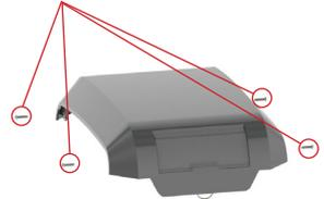
3 Remove both screws to electrical enclosure cover.
