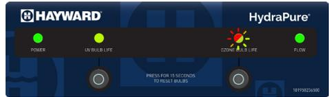
Green or red flashing OZONE BULB LIFE indicates ozone bulb is nearing end of lifespan and will need replacing soon, see page 13
