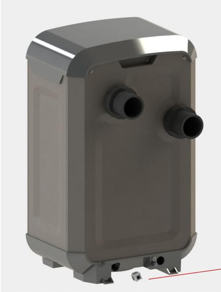
Remove Winterizing O-ring plug near the bottom of the unit by turning counter clockwise. Note, there will be an initial rush of water from the unit after the plug is removed. Allow unit to completely drain, this will take 1-2 minutes. Re-install O-ring plug hand tight.
