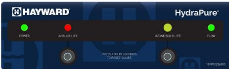
Solid red UV BULB LIFE indicates Lamp is not powered on. Bulbs and ballast should be inspected for proper connection prior to replacement. See page 12
