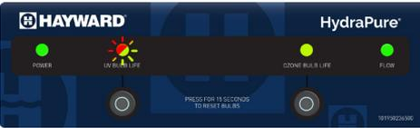
Green or red flashing UV BULB LIFE indicates UV bulb is nearing end of lifespan and will need replacing soon, see page 12
