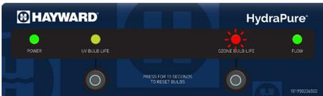
Red flashing OZONE BULB LIFE indicates ozone bulb no longer producing ozone and should be replaced soon.
